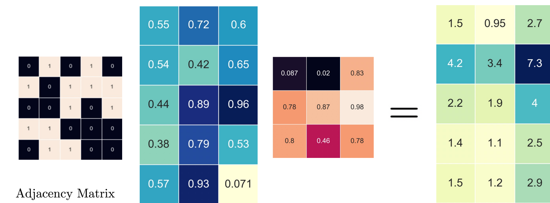
Fig 4: Matrix multiplication showing one layer of a naive GNN.
